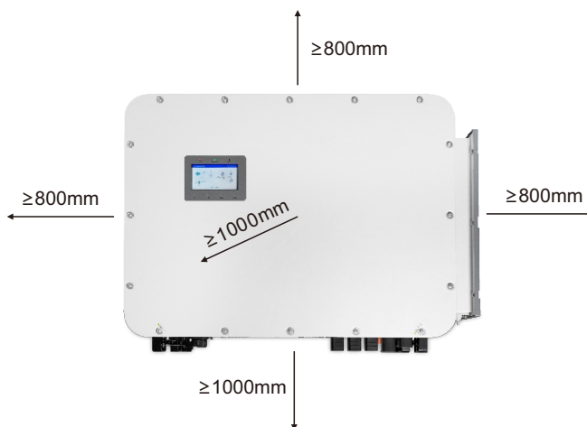
Figure 3.3 Inverter Mounting Clearances
